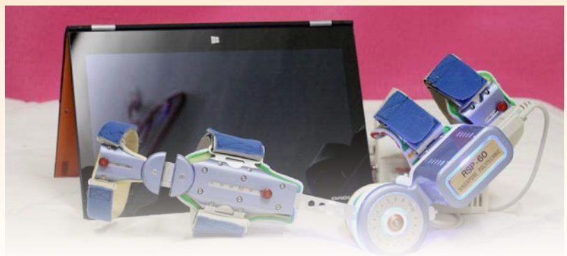
A picture of the Robotics Elbow Brace device 携带式机械手臂的造型
